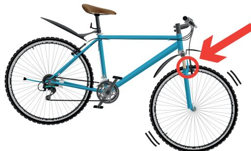
Pulling only the front brake will cause the front wheel to stop and the back wheel to lift off the ground
