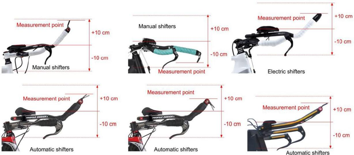
The forearms should also be horizontal and any part of the extension or accessories must be within +/- 10cm of the elbow/forearm supports. For this measurement any moving parts must be placed in the most vertical position.
