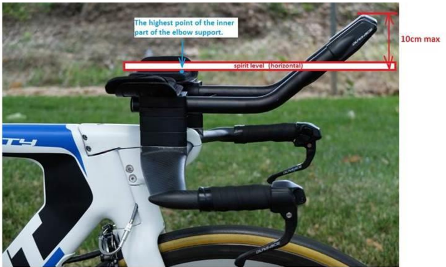
The measuring point on the elbow support is the highest point where the arm is placed.
